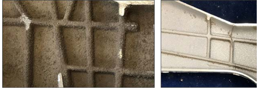
Figure 15: Inner casting surface after cross sectioning of the castings. Left: after removing a non-coated sand core; right: after removing a coated sand core
