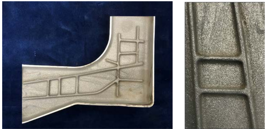
Figure 16: Sand cores with a coating applied by dipping. The coating was furnace dried at 120 °C for 1 h.
