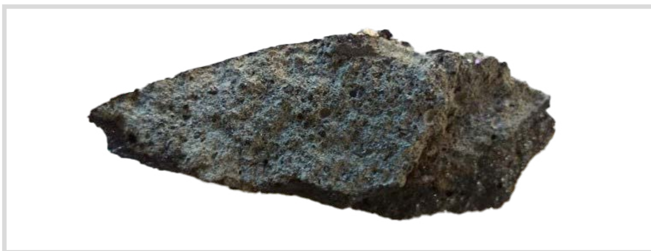
Figure 3: Dosing furnace lining sample
