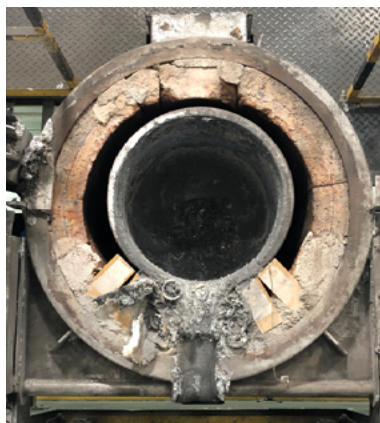
Figure 5: The DURATEK Supermelt after 1284 melt charges.
