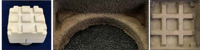
Figure 11: Left: non-coated sand core; middle and right: inner casting surface with significant sand adhesion.
