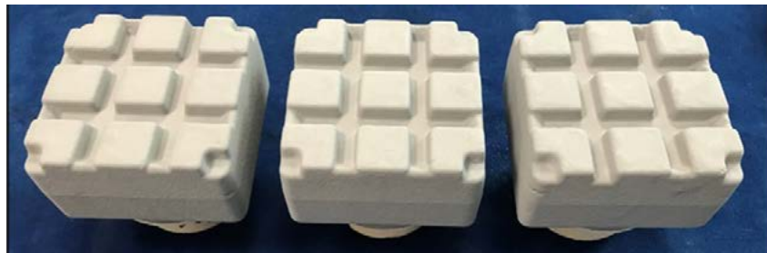
Figure 12: Sand cores with a coating applied by dipping. The coating was furnace dried at 120 °C for 1 h.
