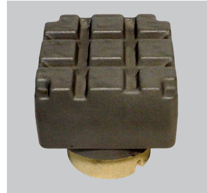
Water-soluble core with applied coating
