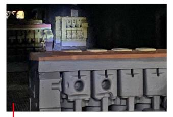
Coated engine block in continuous oven
