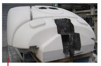
Finished core – 50% faster supplied to moulding line
