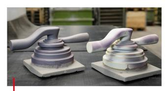
Clearly Visual – Wet vs dry coating layer – the colour change is REVERSIBLE, ie can show moisture pick up
