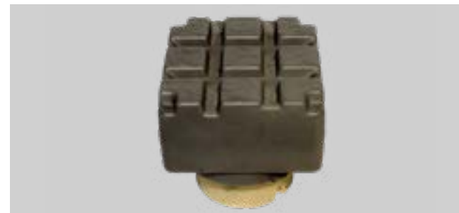
Water-soluble core with applied coating
