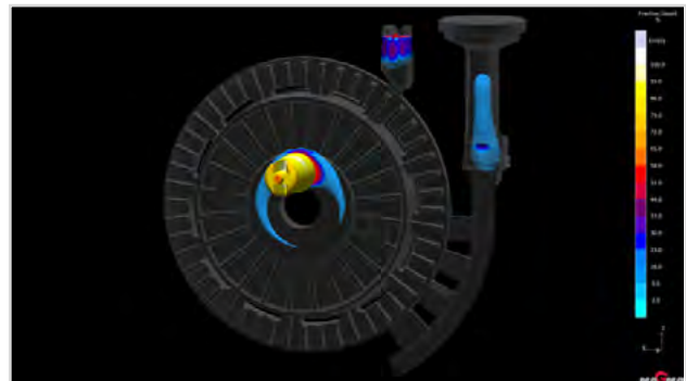
Abb. 11 MAGMA result/ fraction liquid Ansicht
