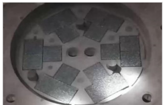
Figure 7. 18 pieces STELEX PrO 150x150x30/10 ppi applied to an iron windmill rotor hub
