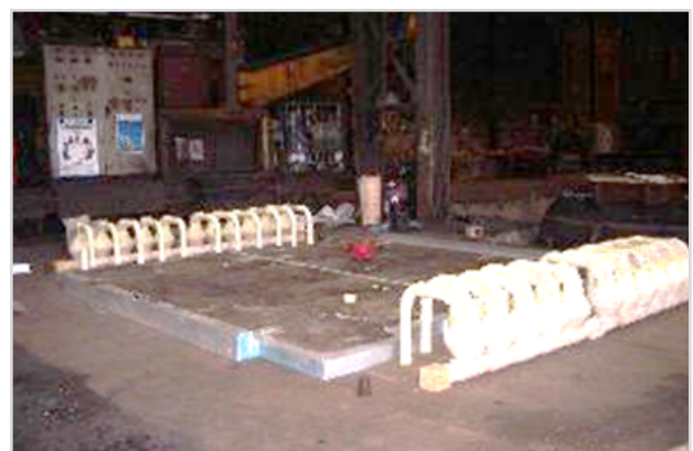
Figure 6. 22 pieces of STELEX ZR applied to a large SG Iron casting requiring Holloware for each filter
