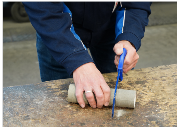
Figure 4. Simple cutting using a hand saw
