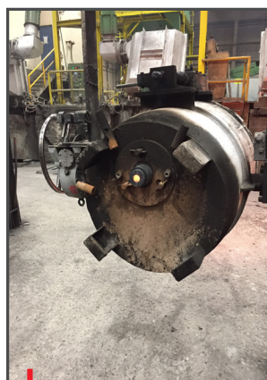
Base nozzle & Pouring nozzle Assembly
