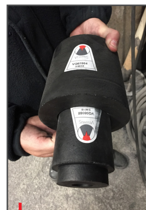
Pouring nozzle change while ladle still hot
