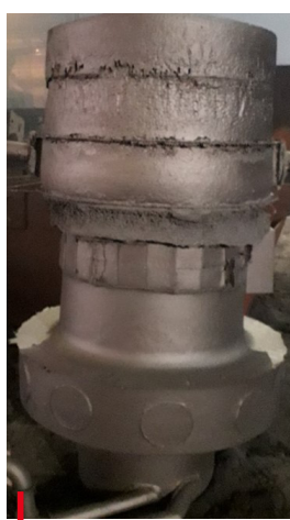
Complete casting picture after shot blasting
