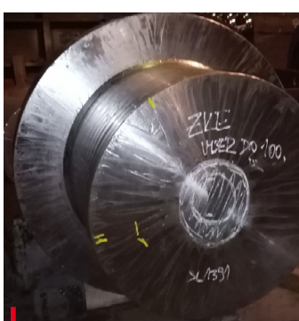
Porosity and segregation identified under the riser by ultrasonic inspection
