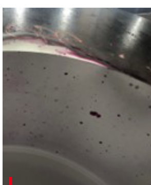
Machining out of both defects under the riser and at the hub in drag until they disappeared before welding followed by additional annealing heat treatment
