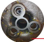
Casting after Magnetic and Ultrasonic inspection. HOLLOTEX CFU
