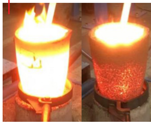
Competitor isopressed crucible (left) and ENERTEK ISO crucible (right) with 1500 °C melt
